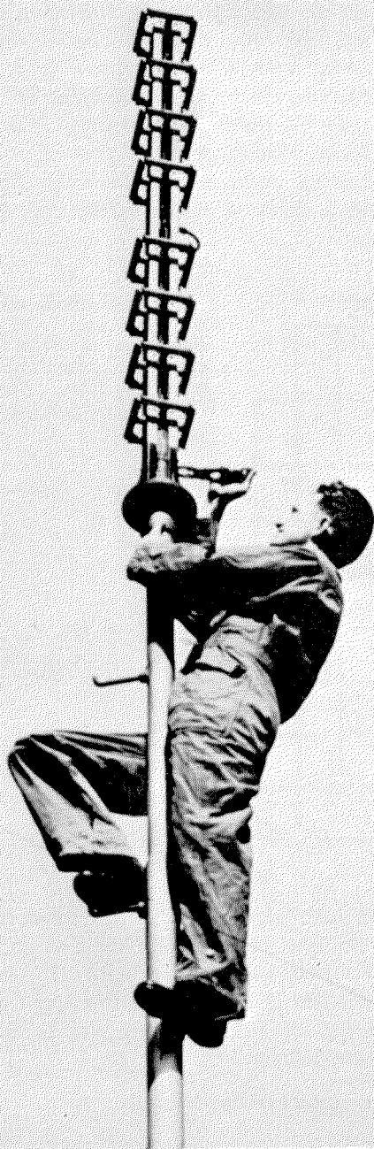
Figure 3—Omnidirectional eight-loop transmitting antenna for the experimental multiplex broadcasting system, located at 67 Broad Street in New York City.
